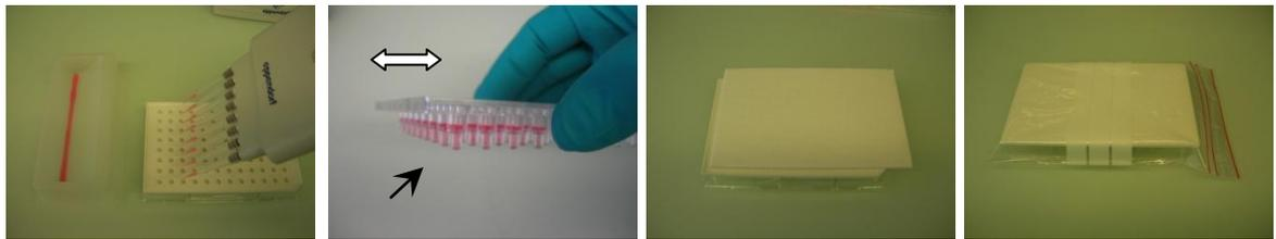
1. Place a new IMAPlate on an empty F-bottomed 96-well plate and pipette 20 µl of capture antibody into the upper compartment of each reaction unit.
