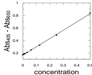
8. Use true absorbance values ( $Abs_{peak} - Abs_{base-line}$ ) to plot the standard curve and calculate the concentration of samples.
