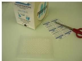
1. Prepare a piece of parafilm (e.g. 100 x 150 mm) and place it on the top of an empty 96-well plate without the wax paper.
