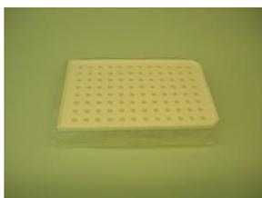
2. Push a new IMAPlate down to the 96-well plate and the parafilm will automatically seal the bottom openings.
