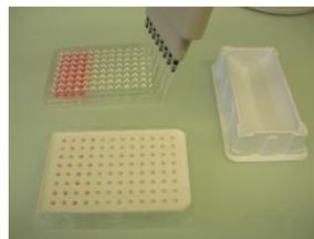
3. Add assay components one by one into the upper compartment. (*Total assay volume\* is recommended between 15  $\mu$ l to 25  $\mu$ l.*)
