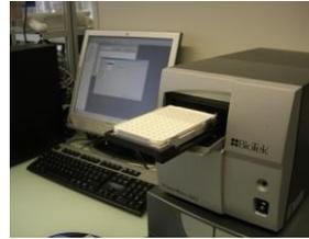
7. Load the IMAPlate adaptor with the assay IMAPlate into the reader and measure both the peak absorbance and base line absorbance.
