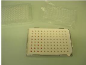
6. Place the IMAPlate in an IMAPlate adaptor and gently tap it in horizontal direction several times to ensure the assay solution filling up the lower compartment.
